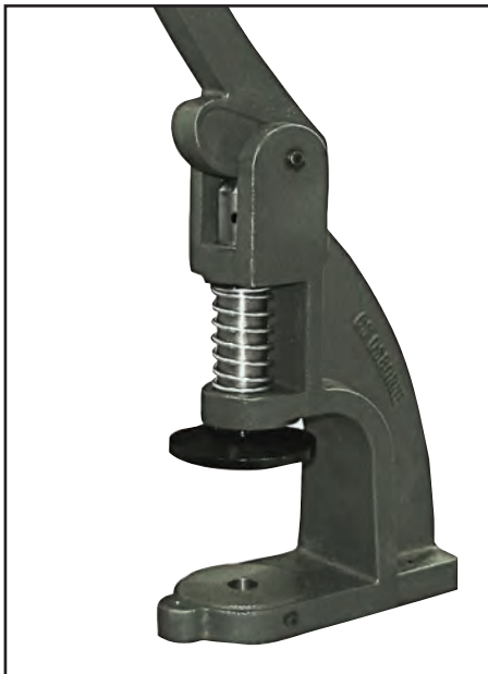
Our Osborne No. W-1 Hand Press Machine also sets SNAPS & VENTILATORS.
